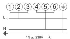
Make sure that the mains characteristics (voltage, nominal, power, etc.) match the ratings indicated on the data plate affixed to the lower right hand cooker upright (remove storage drawer). The cooker is preset for a single-phase earthed electrical connection. It is essential to install a multi-pole circuit breaker that completely disconnects the appliance from the mains, with a minimum contact break distance of 3mm.
